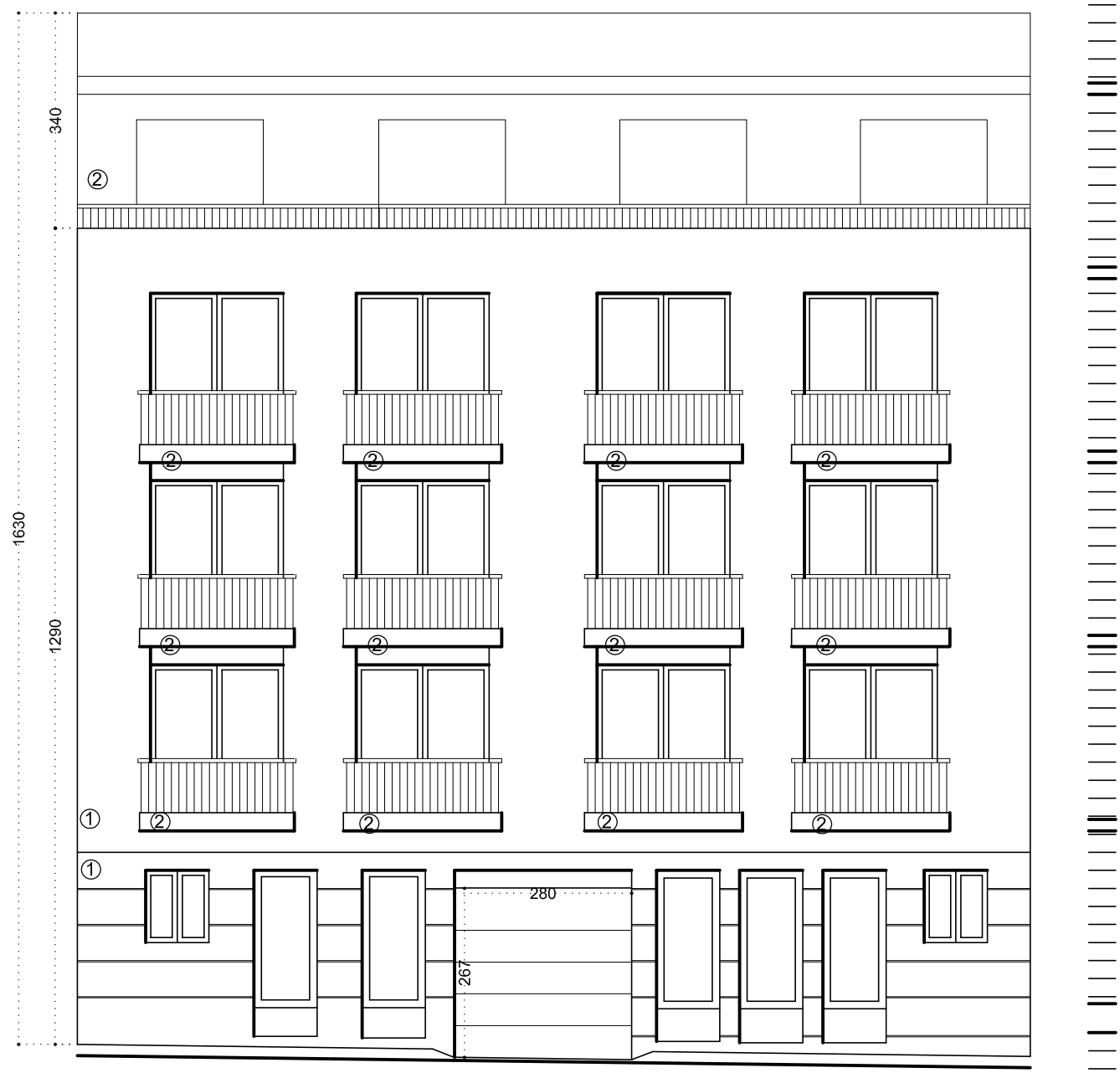
○ Front Elevation Scale 1:100 ① Unpainted Franka Stone ② Painted White Silicato White Aluminium Apertures
